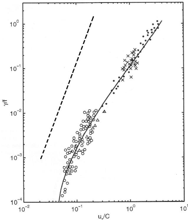
**Figure 3.** Comparison of the experimental data on the wind-induced growth rate  $2\pi\gamma_{in}(\omega)/\omega$  taken from [26] and the damping due to four-wave interactions  $2\pi\Gamma(\omega)/\omega$ , calculated for the narrow in angle spectrum at  $\mu \simeq 0.05$  using equation (6.11) (dashed line).
