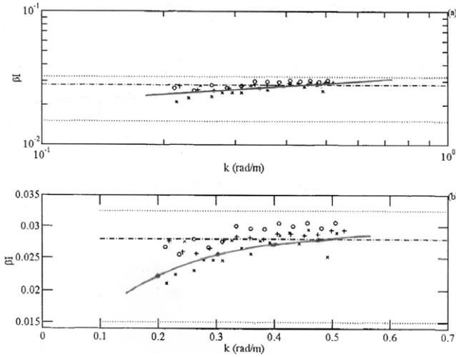
**Figure 2.** Dimensionless wave number spectral coefficient  $\beta_i$  plotted on logarithmic scales (a) and linear scales (b), taken from [20]. Here crosses represent the omnidirectional (averaged by angles) spectrum and dots correspond to  $\xi(k) = 2\beta_i u_* g^{-0.5} k^{-2.5}$ . The solid line in (a) and solid curve in (b) correspond to  $\xi(k) \simeq k^{-7/3}$ .
