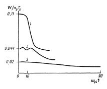
FIG. 2. Time-dependence of the average energy density of the field in the caviton:  $1 \varepsilon / \varepsilon_0 = 6.6$ ; 2: 1.25; 3: 2.7.
