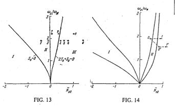
FIG. 13. Phase diagram for the m = 0 mode. Regions I and III correspond to the stable phase; strong auto-oscillations develop in region II. FIG. 14. Phase diagrams for the m = 2 and m = -2 modes. The m = 2 mode is stable in region I and the m = -2 mode in region II.
