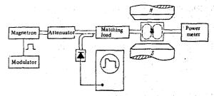
FIG. 3. Schematic illustration of apparatus for the parametric excitation of spin waves.
