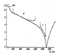
FIG. 15. Weak auto-oscillation threshold vs. constant-magnetic field (YIG sphere,  $M \parallel \langle 100 \rangle$ ).
